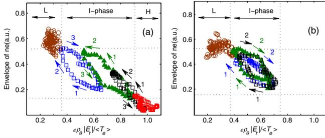
FIG. 3 (color online). Trajectories of the system in phase space of normalized radial electric field  $|E_r|$  and rms of the density envelope (20–100 kHz) measured at  $\Delta r = -5$  mm for shots I (a) and II (b).
