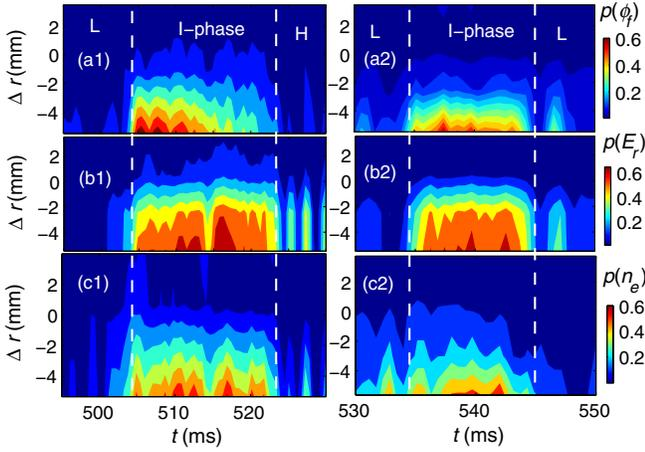
FIG. 5 (color online). Spatio-temporal distributions of amplitudes of fluctuating floating potential  $\delta\phi$  (a1 and a2), radial electric field  $\delta E_r$  (b1 and b2), and electron density  $\delta n_e$  (c1 and c2) of frequency  $f \approx 2-3$  kHz for shots I and II.
