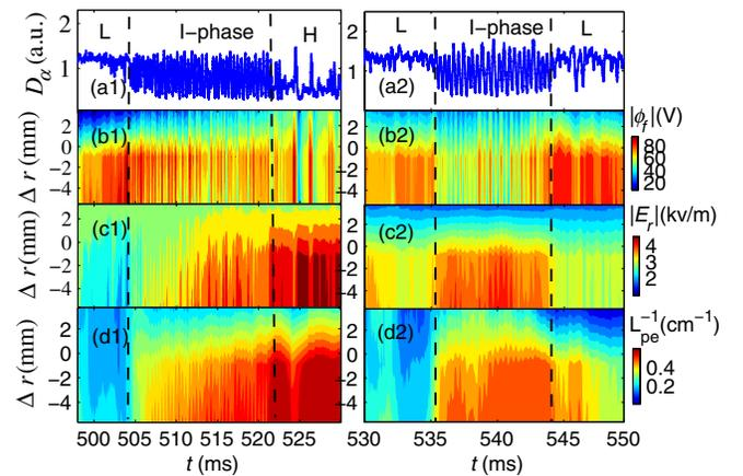
FIG. 2 (color online). Time evolutions of  $D_\alpha$  signals [(a1) and (a2)], the spatio-temporal distributions of the amplitudes of the floating potential  $|\phi_f|$  [(b1) and (b2)] radial electric field  $|E_r|$  [(c1) and (c2)], and the inverse scale lengths of electron pressure gradients  $L_{pe}^{-1}$  [(d1) and (d2)] for shots I and II.
