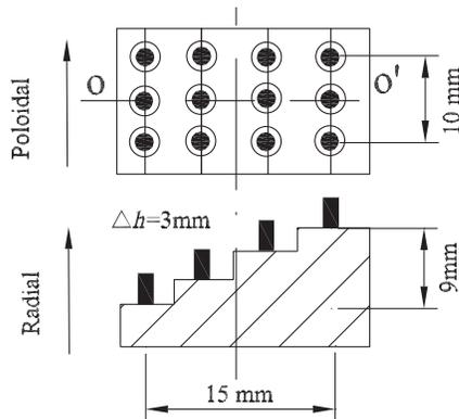
FIG. 1. Sketch of the four-step probe array.
