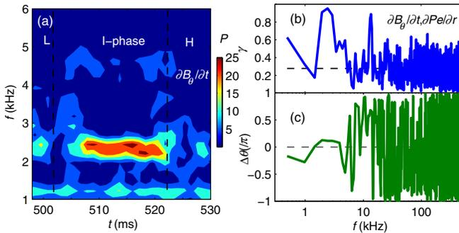
FIG. 6 (color online). Time evolutions of the spectrum of  $\partial B_\theta/\partial t$  (a), the spectra of coherence  $\gamma$  (b) and phase shift (c) between  $\partial B_\theta/\partial t$  and the gradient of electron pressure  $\partial p_e/\partial r$  for shot I.
