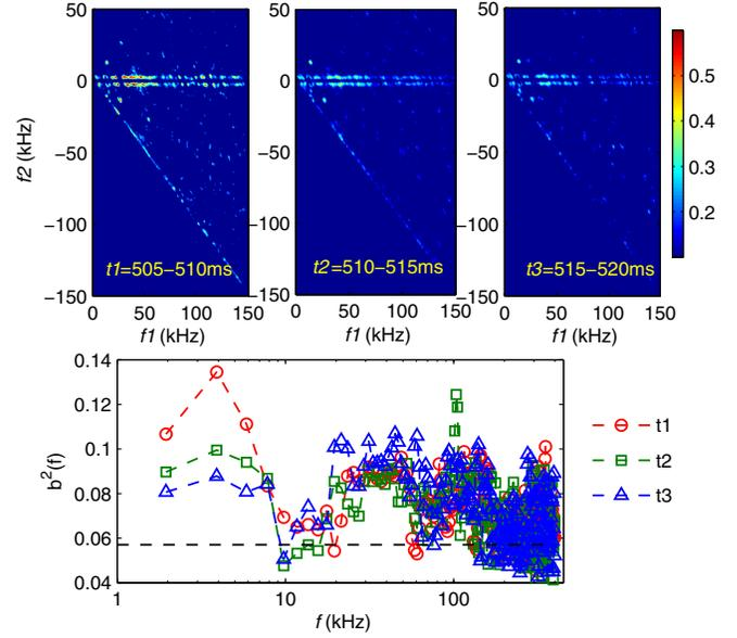
FIG. 4 (color online). Bicoherence spectra estimated in 505–510 ms (a), 510–515 ms (b) and 515–520 ms (c), and the corresponding summed bicoherence spectra (d) in shot I.
