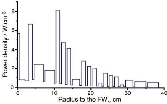
Fig. 3. Radial power density distribution in the blanket module as a function of distance from the first wall in the radial direction.
