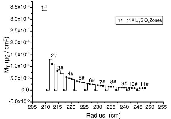
Fig. 4. Tritium distribution vs. the blanket thickness.
