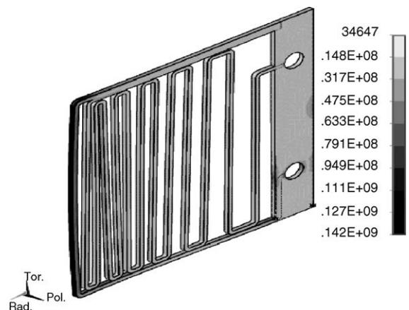
Fig. 8. 3-D stress distribution of cooling tube (Pa).
