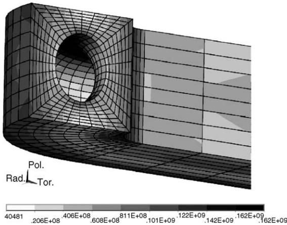
Fig. 9. Stress distribution in the first wall (Pa).
