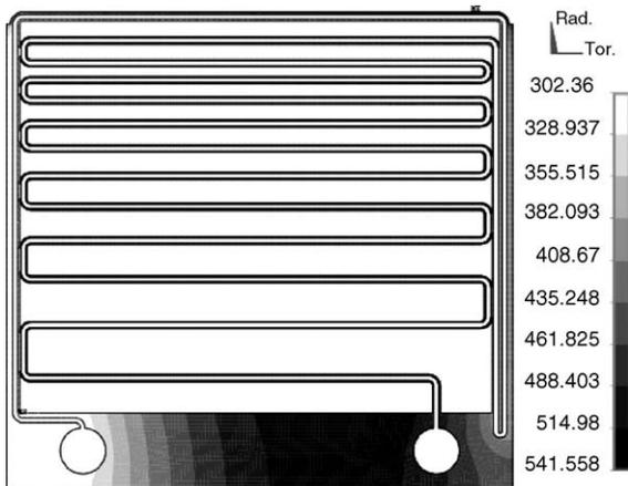
Fig. 7. Temperature distribution of cooling plate (°C).
